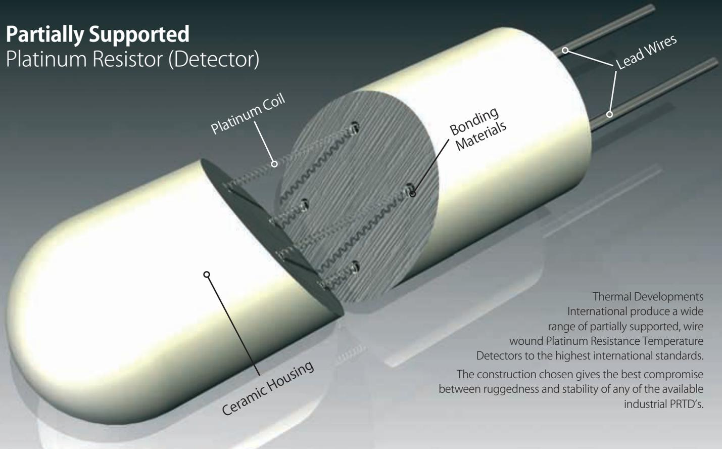
Thermal Developments International produce a wide range of partially supported, wire wound Platinum Resistance Temperature Detectors to the highest international standards. The construction chosen gives the best compromise between ruggedness and stability of any of the available industrial PRTD's.
